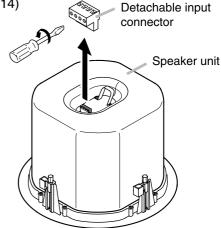
**2-2.** Insert the stripped cable end into the terminal and tighten the terminal screw with a screwdriver.
