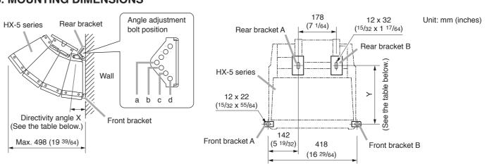
Note: The angle X and the distance Y vary depending on the bolt position.
