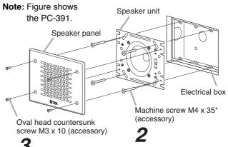
\* When using an electrical box other than our YC-150 or YC-150E, use screws that are appropriate for that electrical box.
